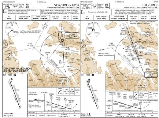
'attached' to a specific runway, you would effectively enter a right traffic pattern as you overfly the runway and land after flying the right-hand traffic pattern (see the diagram below).
